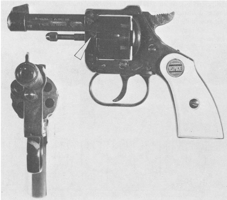
FIG. 1—Rosco Vestpocket .22 caliber six-shot revolver, barrel length 2\frac{1}{4} in. Note the marks on the frame of the gun produced by the bullet discharged from the cylinder chamber (arrow). The insert shows the front view of the gun and the position of the cylinder at the time of discharge. The frame causes a half-moon-like obstruction of the cylinder chamber, and is the object which is responsible for "shaving" the bullet.
